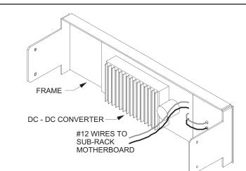
The DC to DC converters provide a regulated +13.8 Vdc to the output terminals over a wide range of DC input voltages. Valuable rack space has been saved by mounting the DC to DC converter inside the rear panel frame that attaches to the rear of the subrack. A terminal block is located on the outside of the subrack rear panel for the DC input voltage. The DC to DC converters comes in two different models.
